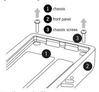
Note that you should not attempt to remove the PTT keypad before removing the front panel from the chassis. See "Replacing the PTT keypad" on page D-8 for more information.
