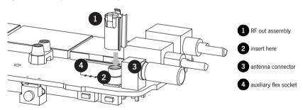
Figure D-11: Placing the RF out assembly
