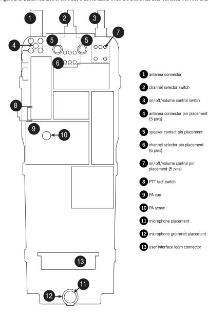
Figure D-9: Top surface of PCB, which is visible only when the PCB has been removed from the chassis
